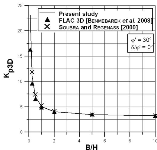
Fig. 12 – Comparison between solutions by BENMEBAREK *et al.* [2008], by SOUBRA and REGENASS [2000] and by the proposed model, in the case  $\delta/\varphi'=0$  and for  $\varphi'=30^\circ$ .
