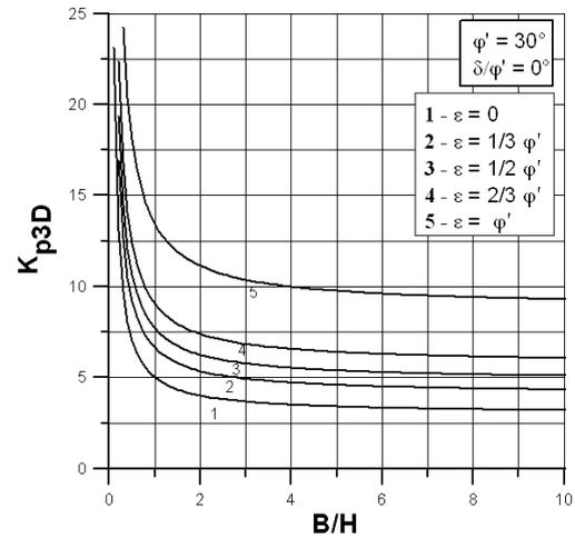
Fig. 21 – Passive earth pressure coefficient  $K_{p3D}$  coefficient versus  $B/H$  for different slope angles  $\varepsilon$ , in the case  $\delta/\varphi'=0$  and for  $\varphi'=30^\circ$ .
