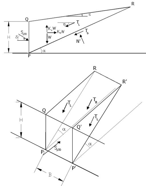
Fig. 2 – Three-dimensional model for the analysis of passive earth pressure coefficient; a) cross section; b) Three-dimensional view.
