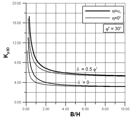
Fig. 3 –  $K_{p3D}$  versus  $B/H$  for two different values of  $\eta$ , in the case  $\delta/\varphi'=0$  and  $\delta/\varphi'=0,5$ .
