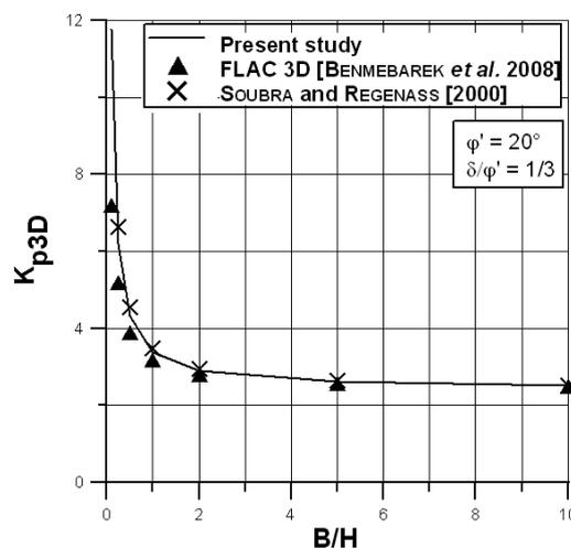
Fig. 14 – Comparison between solutions by BENMEBAREK *et al.* [2008], by SOUBRA and REGENASS [2000] and by the proposed model, in the case  $\delta/\varphi'=1/3$  and for  $\varphi'=20^\circ$ .
