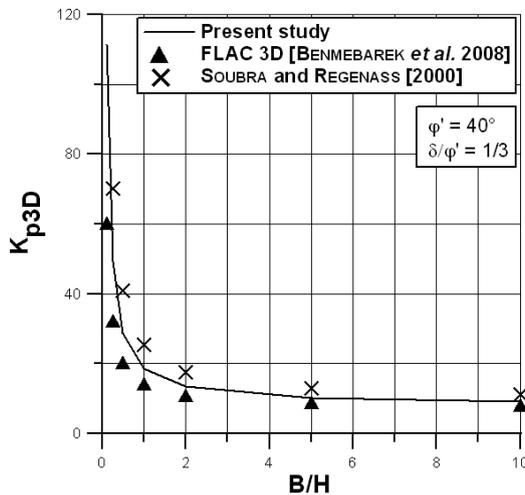
Fig. 16 – Comparison between solutions by BENMEBAREK *et al.* [2008], by SOUBRA and REGENASS [2000] and by the proposed model, in the case  $\delta/\varphi'=1/3$  and for  $\varphi'=40^\circ$ .
