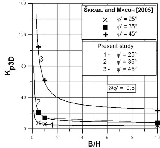
Fig. 9 –  $K_{p3D}$  versus  $B/H$  in the case  $\delta/\phi' = 0.5$ , for three different values of the friction angle:  $\phi' = 25^\circ$   $\phi' = 35^\circ$   $\phi' = 45^\circ$ : comparison between SKRABL and MACHU [2007] solution and the proposed one.
