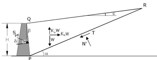
Fig. 1 – KAPILA [1962] model for the analysis of passive earth pressure in pseudo-static conditions.
