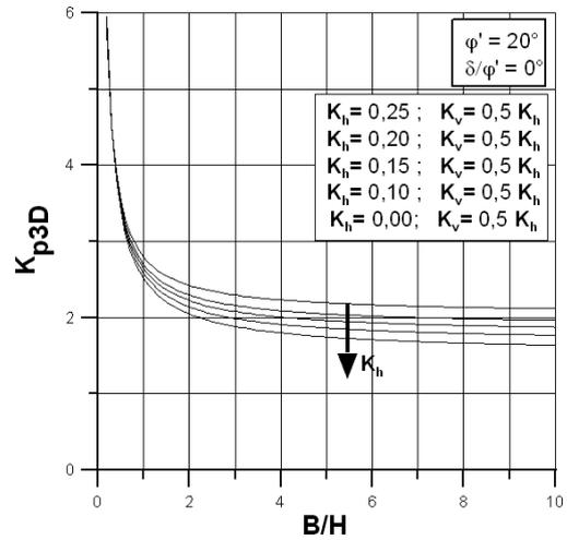
Fig. 17 – Seismic passive earth pressure coefficient  $K_{p3D}$  coefficient versus  $B/H$  for different seismic horizontal coefficient  $K_h$  in the case  $\delta/\varphi'=0$  and for  $\varphi'=20^\circ$ .
