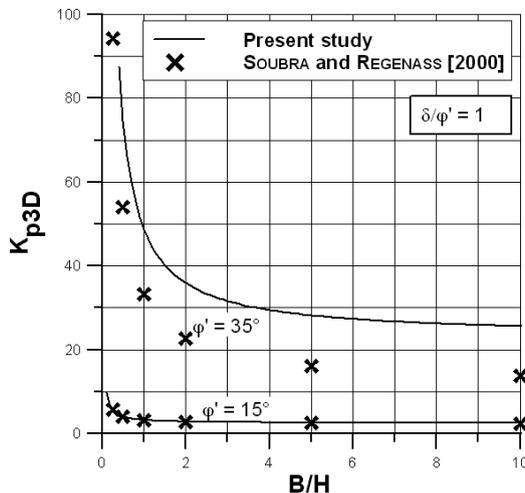
Fig. 8 –  $K_{p3D}$  versus  $B/H$  in the cases  $\phi' = 15^\circ$  and  $\phi' = 35^\circ$ : comparison between SOUBRA and REGENASS 2000] solution and the proposed one ( $\delta/\phi' = 1$ ).
