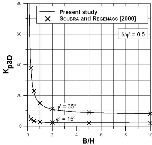
Fig. 7 –  $K_{p3D}$  versus  $B/H$  in the cases  $\phi' = 15^\circ$  and  $\phi' = 35^\circ$ : comparison between SOUBRA and REGENASS [2000] solution and the proposed one ( $\delta/\phi' = 0.5$ ).
