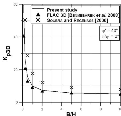
Fig. 13 – Comparison between solutions by BENMEBAREK *et al.* [2008], by SOUBRA and REGENASS [2000] and by the proposed model, in the case  $\delta/\varphi'=0$  and for  $\varphi'=40^\circ$ .
