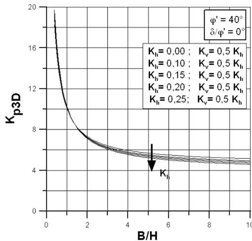
Fig. 19 – Seismic passive earth pressure coefficient  $K_{p3D}$  coefficient versus  $B/H$  for different seismic horizontal coefficient  $K_h$  in the case  $\delta/\varphi'=0$  and for  $\varphi'=40^\circ$ .
