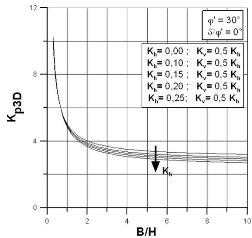
Fig. 18 – Seismic passive earth pressure coefficient  $K_{p3D}$  coefficient versus  $B/H$  for different seismic horizontal coefficient  $K_h$  in the case  $\delta/\varphi'=0$  and for  $\varphi'=30^\circ$ .
