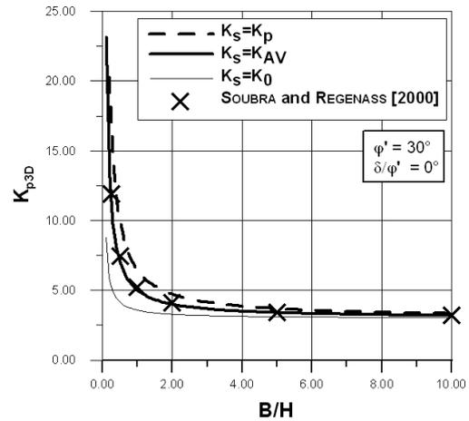
Fig. 5 –  $K_{p3D}$  versus  $B/H$  for different  $K_s$  values, ( $K_s = K_0$ ;  $K_s = K_{AV}$ ;  $K_s = K_p$ ), in the case  $\phi'=30^\circ$  and  $\delta/\phi'=0$ .
