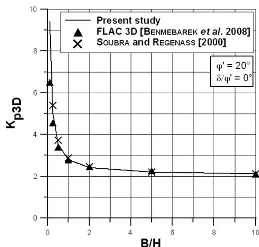
Fig. 11 – Comparison between solutions by BENMEBAREK *et al.* [2008], by SOUBRA and REGENASS [2000] and by the proposed model, in the case  $\delta/\varphi'=0$  and for  $\varphi'=20^\circ$ .
