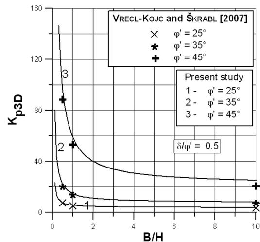
Fig. 10 –  $K_{p3D}$  versus  $B/H$  in the case  $\delta/\phi' = 0.5$ , for three different values of the friction angle:  $\phi' = 25^\circ$   $\phi' = 35^\circ$ ,  $\phi' = 45^\circ$ : comparison between VRECL-KOJC and SKRABL [2007] solution and the proposed one.
