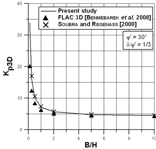
Fig. 15 – Comparison between solutions by BENMEBAREK *et al.* [2008], by SOUBRA and REGENASS [2000] and by the proposed model, in the case  $\delta/\varphi'=1/3$  and for  $\varphi'=30^\circ$ .
