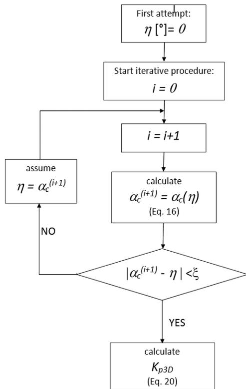
Fig. 4 – Flow chart for the determination of  $\eta$  and  $K_{p3D}$ .
