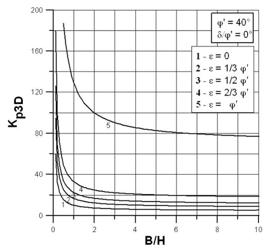
Fig. 22 – Passive earth pressure coefficient  $K_{p3D}$  coefficient versus  $B/H$  for different slope angles  $\varepsilon$ , in the case  $\delta/\varphi'=0$  and for  $\varphi'=40^\circ$ .
