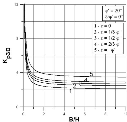
Fig. 20 – Passive earth pressure coefficient  $K_{p3D}$  coefficient versus  $B/H$  for different slope angles  $\varepsilon$ , in the case  $\delta/\varphi'=0$  and for  $\varphi'=20^\circ$ .
