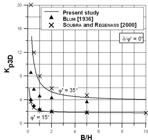
Fig. 6 –  $K_{p3D}$  versus  $B/H$  in the cases  $\phi'=15^\circ$  and  $\phi'=35^\circ$ : comparison between BLUM [1932] solution, SOUBRA and REGENASS [2000] solution and the proposed one ( $\delta/\phi'=0$ ).
