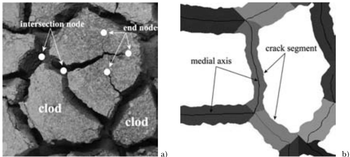
Fig. 2 – Crack pattern: a) typical original crack pattern obtained during drying; b) typical crack pattern after image processing.
