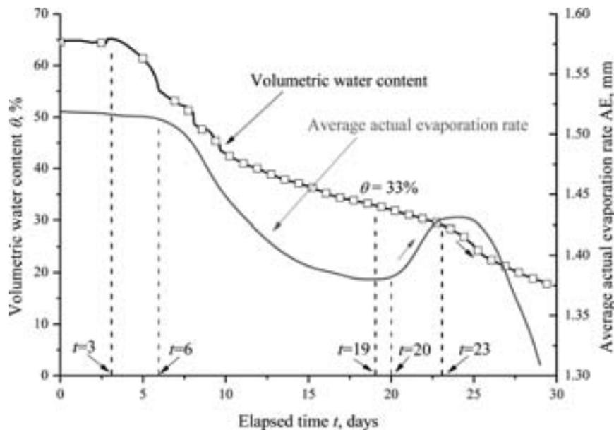
Fig. 6 – Variations of volumetric water content at 50 mm depth and average actual evaporation rate.
