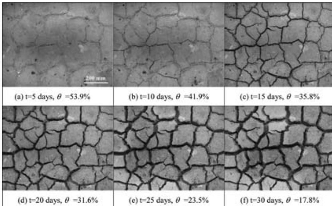
Fig. 8 – Evolution of crack patterns during drying.
