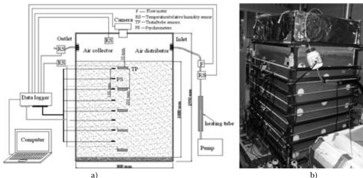
Fig. 1 – Schematic drawing a) and a photo of the environmental chamber b).
