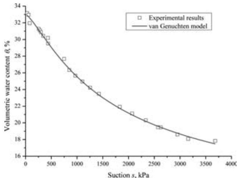
Fig. 7 – Suction and volumetric water content measured at 50 mm depth during drying.
