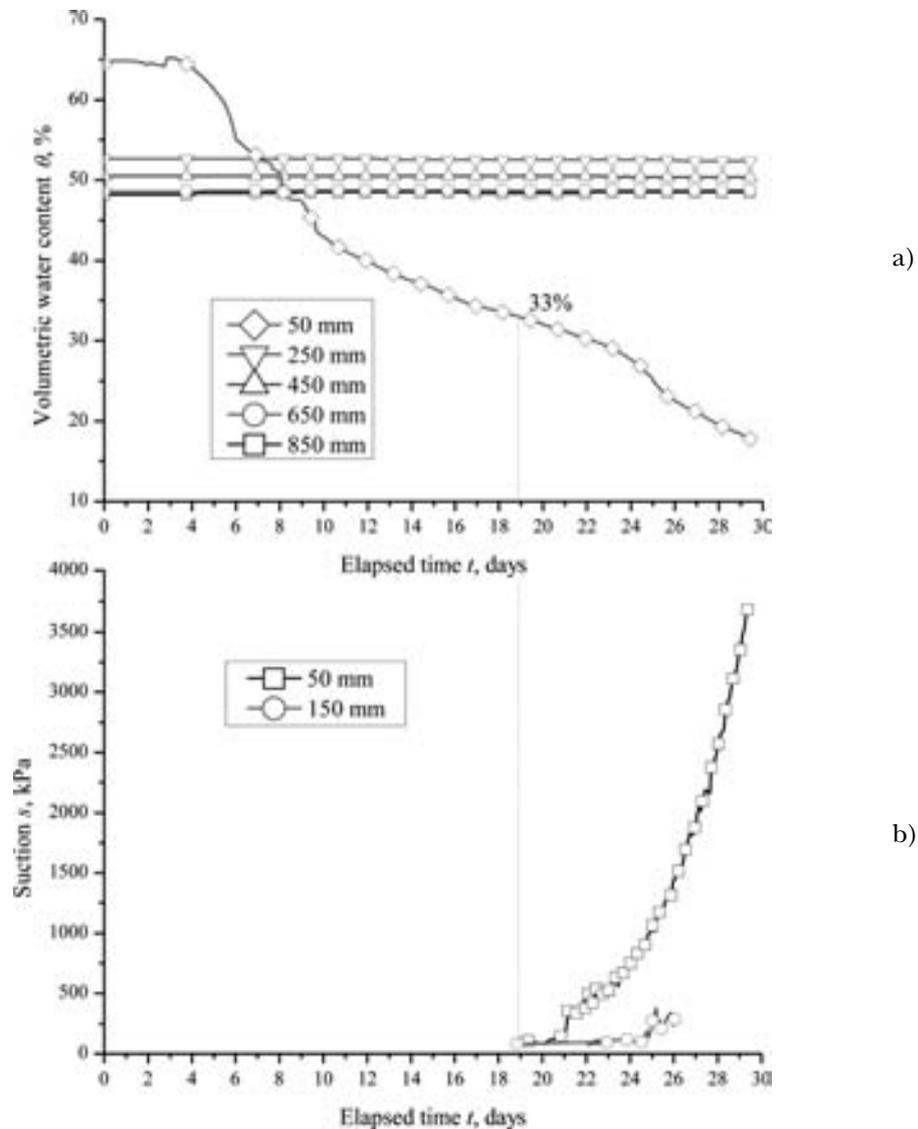
Fig. 5 – Variations of soil volumetric water content a) and soil suction b).
