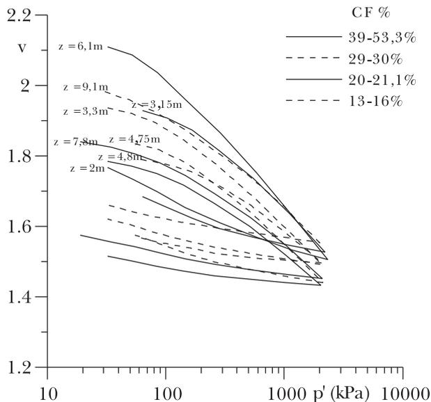
Fig. 5 – Summary of the oedometer tests.
