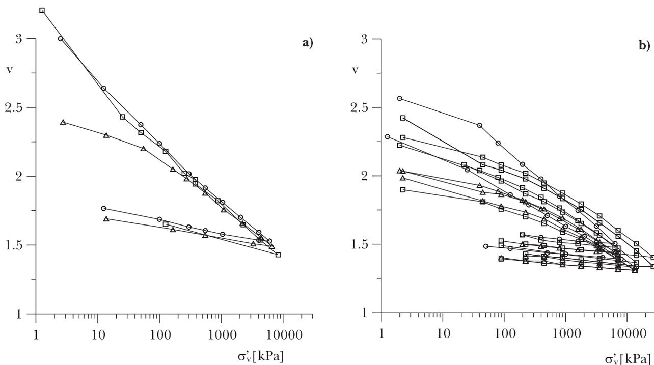
Fig. 1 – Oedometric compression test data for reconstituted samples of Po River embankment silts (a) 45% clay content (b) 8% clay content [after NOCILLA *et al.*, 2006].
