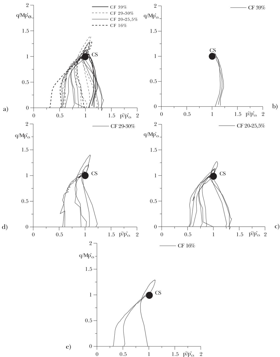
Fig. 10 – Normalised shearing paths for the triaxial tests. (a) Summary Plot; (b) 39% clay content; (c) 29-30% clay content; (d) 20-25.5% clay content; (e) 16% clay content.
