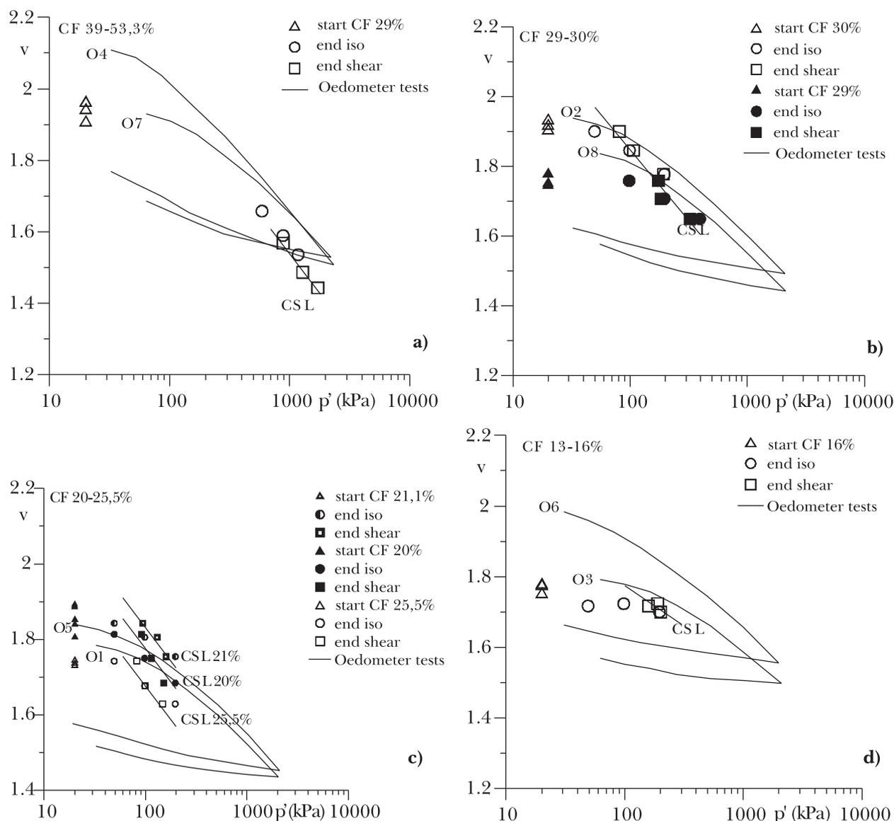
Fig. 7 – Triaxial and oedometer data. (a) 39-53.3% clay content (b) 29-30% clay content (c) 20-25.5% clay content (d) 13-16% clay content.
