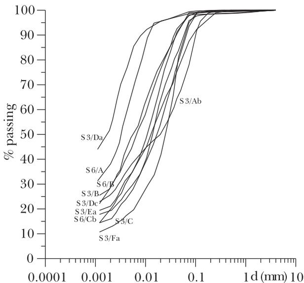
Fig. 4 – Grading curves for the soils (data from A.I.P.O., 2004).
