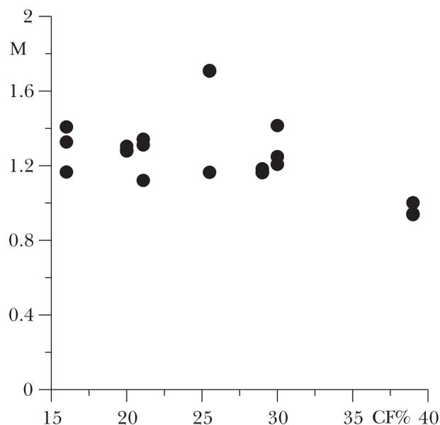
Fig. 9 – The influence of clay fraction on the Critical State Line gradient, M.
