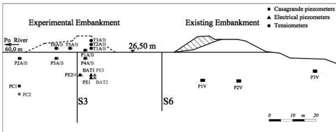
Fig. 3 – Schematic section illustrating borehole and instrumentation locations.
