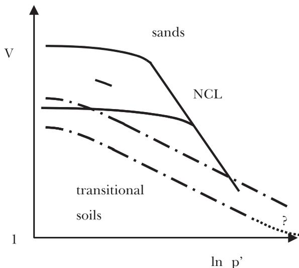
Fig. 2 – Schematic illustration of the compression of sands and “transitional” soils [after NOCILLA *et al.*, 2006].
