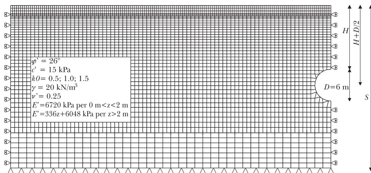
Fig. 6 - Typical density of the meshes used and numerical values for the physical and mechanical parameters of the soil.
