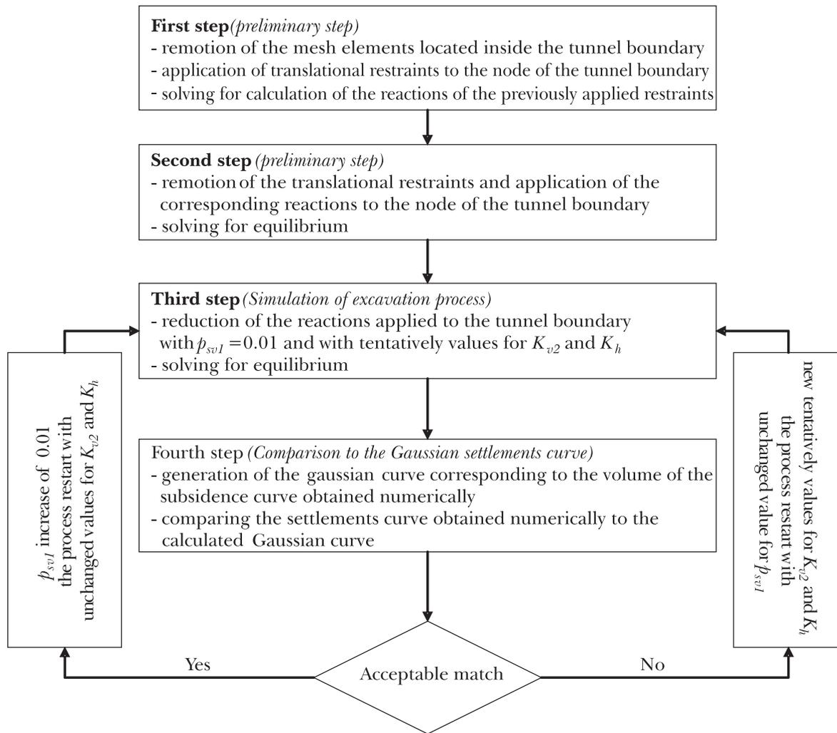
Fig. 3b - Steps for the application of the stress release technique.
