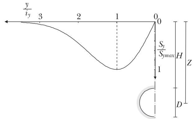
Fig. 2 - Normalized superficial horizontal displacements.
