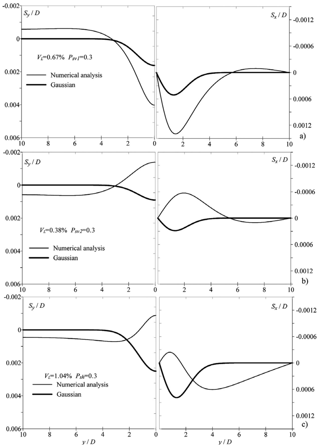
Fig. 4 - Effects of the reduction of the individual components of the force ( $H=12$  m,  $D=6$  m  $S=42$  m and  $k_0=0.5$ ).
