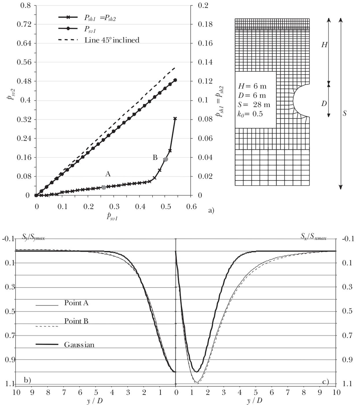
Fig. 5 - Surface displacements obtained using the differential release technique.
