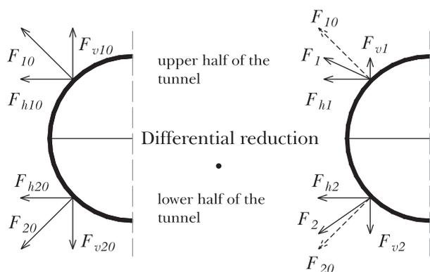
Fig. 3a - Differential reduction of the forces acting on the tunnel boundary.
