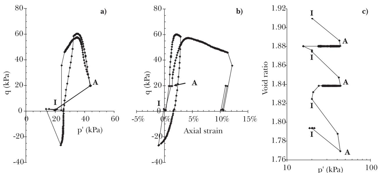
Fig. 6 – a)  $q$  vs  $p'$  stress path, b)  $q$  vs axial strain and c) void ratio vs  $p'$  in Test BN10.
