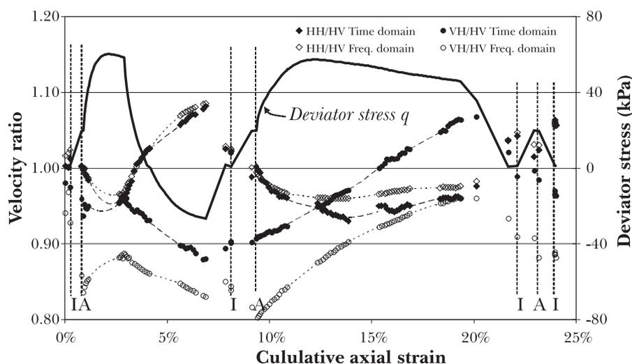
Fig. 9 – Variation of anisotropy of shear wave velocity comparing time domain and frequency domain through test BN10.
