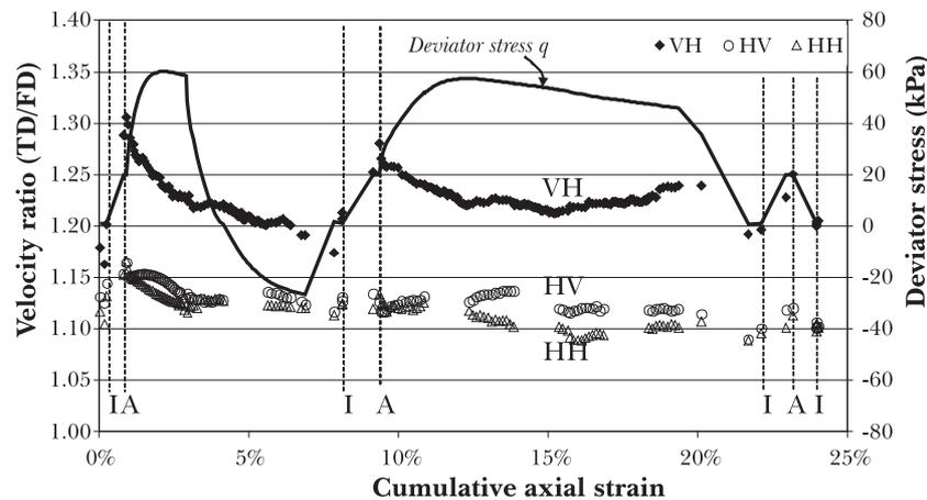
Fig. 8 – Variation of velocity ratios comparing time domain (TD) and frequency domain (FD) through test BN10.
