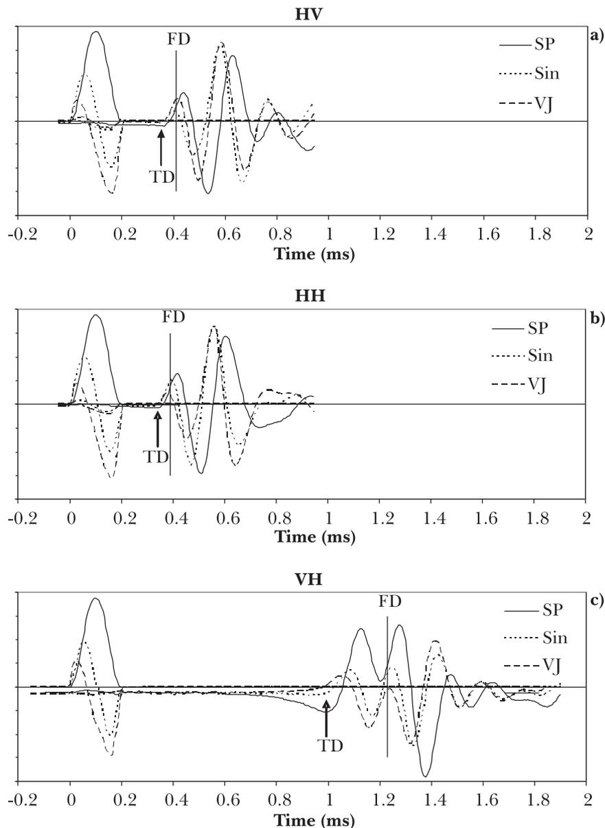
Fig. 3 – Pulse readings on reconstituted sample of Bothkennar clay: “normalised voltages” for a) *hv* b) *hh* and c) *vh* directions.
