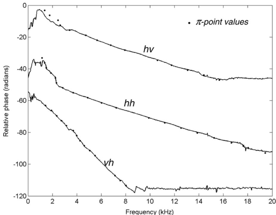
Fig. 5 – Unwrapped phase compared with  $\pi$ -point measurements.
