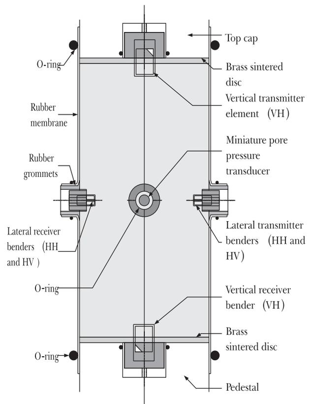
Fig. 1 – Bender element mountings for  $vh$ ,  $hv$  and  $hh$  directions.
