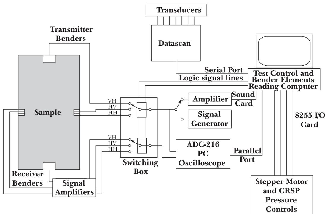
Fig. 2 – Schematic diagram of bender data acquisition system.
