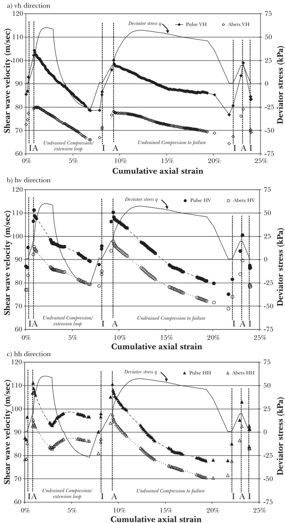
Fig. 7 – Variation of shear wave velocities and deviator stress during test BN10 in a) vh direction, B) hv direction, and c) hh direction.
