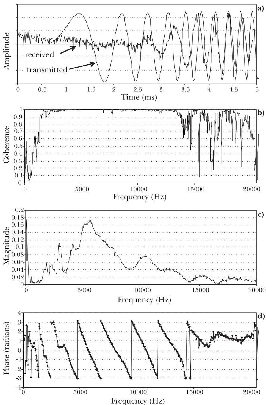
Fig. 4 – a) start of frequency-sweep signal, b) coherence, c) magnitude and d) phase for system transfer function (Test BR4  $lv$  direction).
