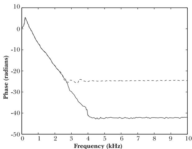
Fig. 14 – Phase delay estimation with crosstalk (dashed line) and with crosstalk removed (solid line) (76mm tall, 75mm wide sample).
