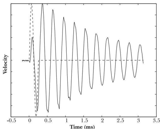
Fig. 8 – Response of bender in air subjected to 4kHz single cycle excitation.
