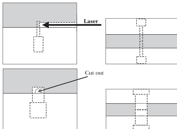
Fig. 5 – Polyurethane samples: cutout for laser (left) and tip to tip configuration (right).
