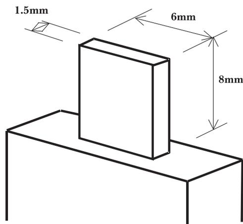
Fig. 4 – Dimensions of UCL bender.
