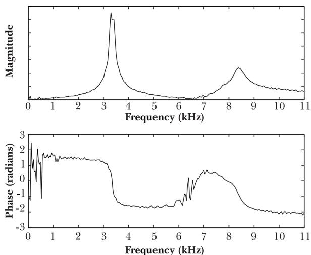
Fig. 7 – Magnitude and phase of transfer function estimate of lateral response of free bender element.
