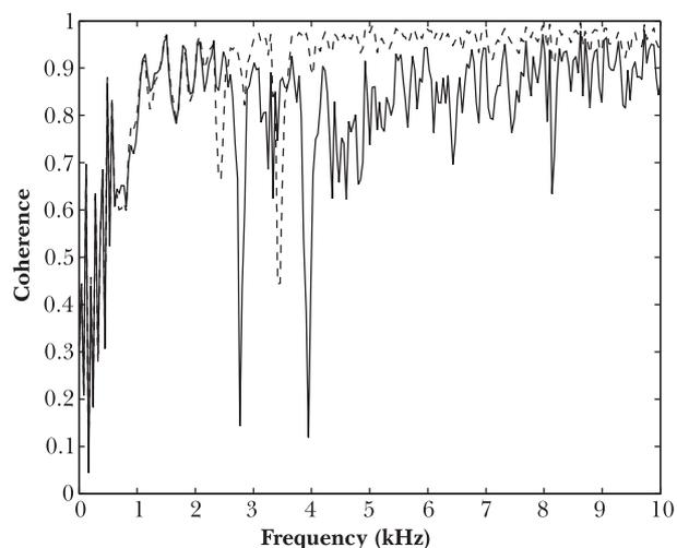
Fig. 15 – Coherence of transfer function for 76mm long, 75mm diameter sample with and without crosstalk removed.
