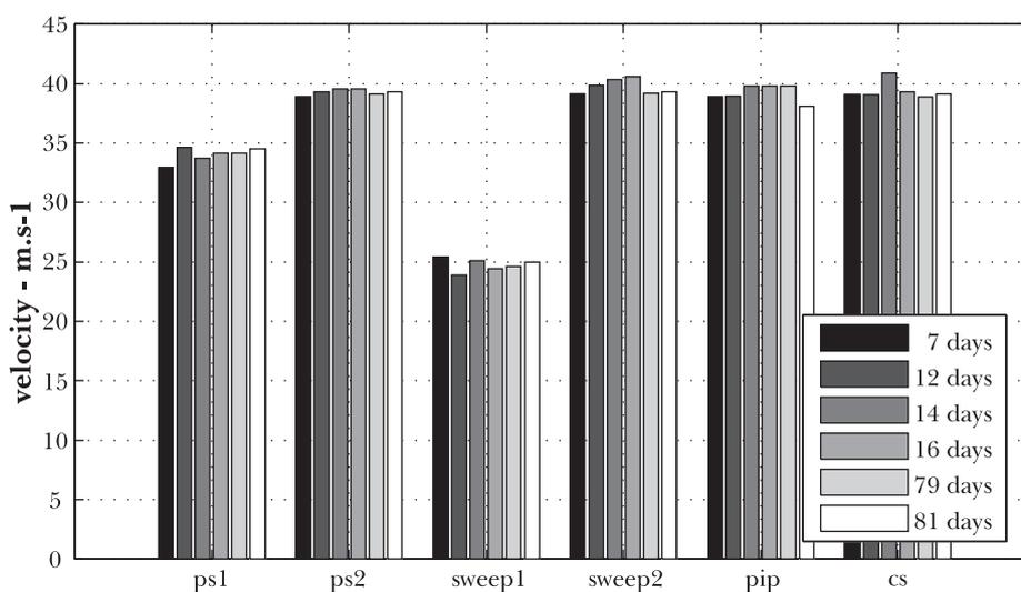
Fig. 3 – Repeatability test showing how estimate of shear wave velocity varies in a single sample in 6 different testing conditions.
