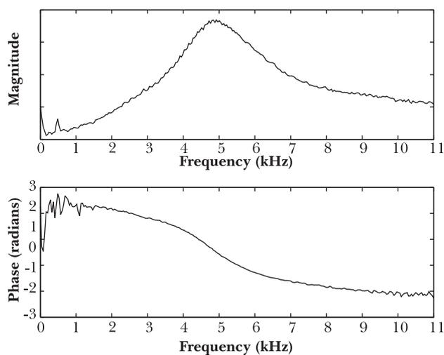
Fig. 9 – Magnitude and phase of transfer function estimate of lateral response of free bender element mounted in polyurethane sample.
