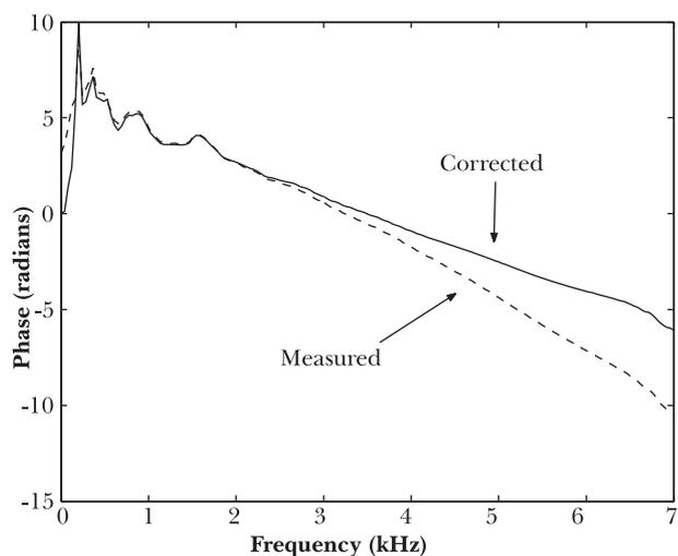
Fig. 6 – Phase delay plot corrected for instrumentation phase delay – short transmission distance.
