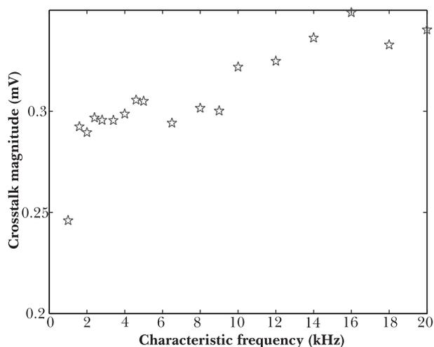
Fig. 13 – Variation in crosstalk with characteristic frequency of pulse transmitted signal.
