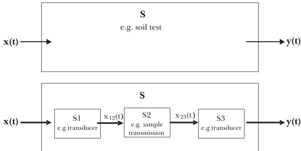
Fig. 1 – Dynamical system schemes for bender element testing.
