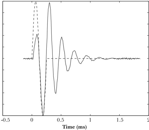
Fig. 10 – Response of bender in polyurethane sample subjected to 4kHz single cycle excitation.
