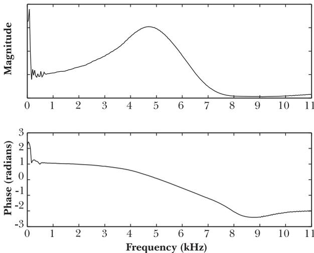
Fig. 11 – Magnitude and phase of transfer function estimate of bender transmitter and receiver touching tip to tip and surrounded by polyurethane.
