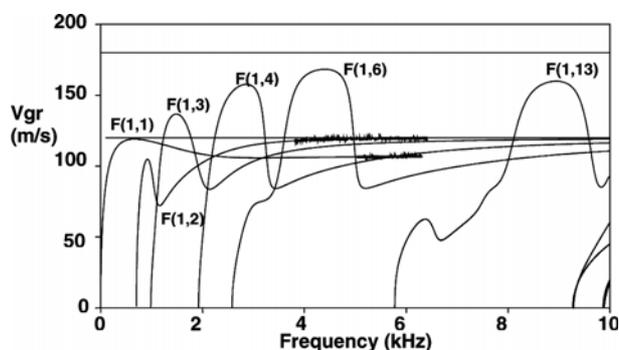
Fig. 9 – Group velocity curves of various flexural modes of an elastic cylinder of  $r = 5$  cm;  $v_s = 120$  m/s;  $\nu = 0.1$ .
