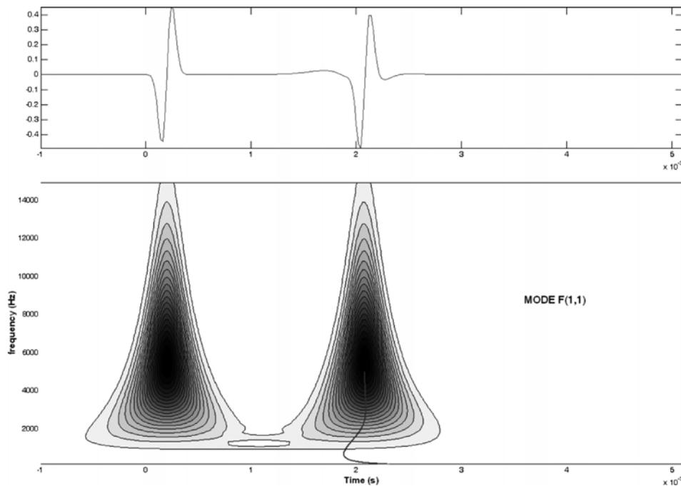
Fig. 10 – Wavelet analysis of a signal numerically propagated in a cylinder. Cylinder properties  $V_s = 120$  m/s  $\nu = 0.1$ , radio 5 cm. Gabor wavelet with  $\sigma = 1$  and  $\eta = 5$ .
