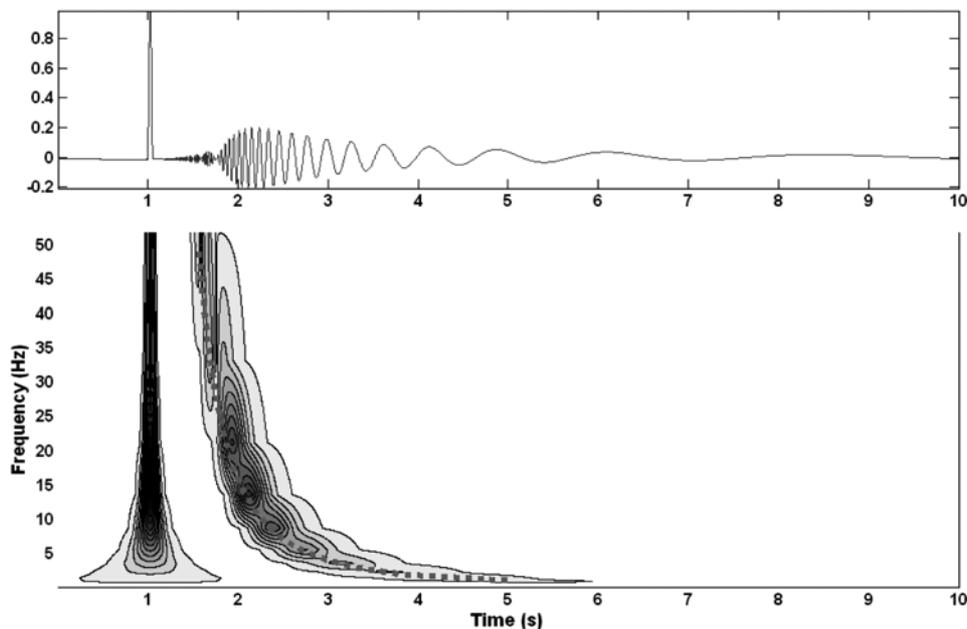
Fig. 8 – Dispersive propagation of a pulse (above) and normalised scalogram (below). Gabor wavelet with  $\sigma = 1$  and  $\eta = 5$ .
