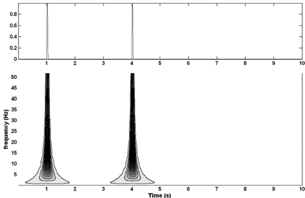
Fig. 7 – Non-dispersive propagation of a pulse signal (above) and normalised scalogram (below). Gabor wavelet with  $\sigma = 1$  and  $\eta = 5$ .
