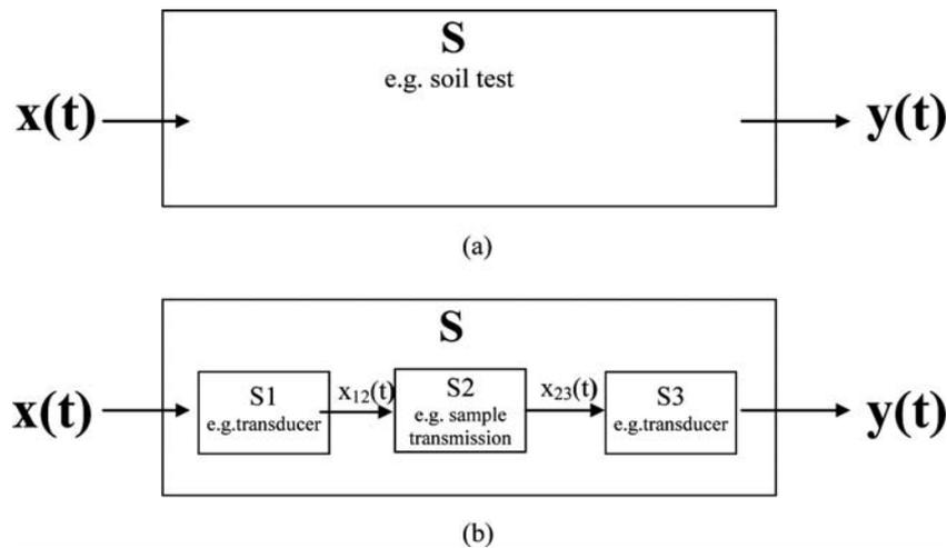
Fig. 1 – Dynamic systems for modelling seismic soil testing (a) without and (b) with internal sub-systems.
