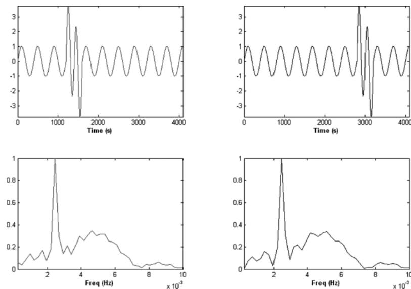
Fig. 4 – Two different transient signals (above) and their identical amplitude spectra (below).
