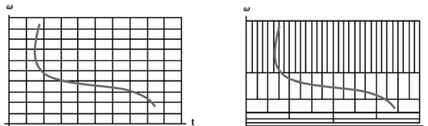
Fig. 5 – Schematic localization on the time-frequency plane of a base of windowed harmonics (left) and a wavelet base (right). Adapted from HARROP [2004].
