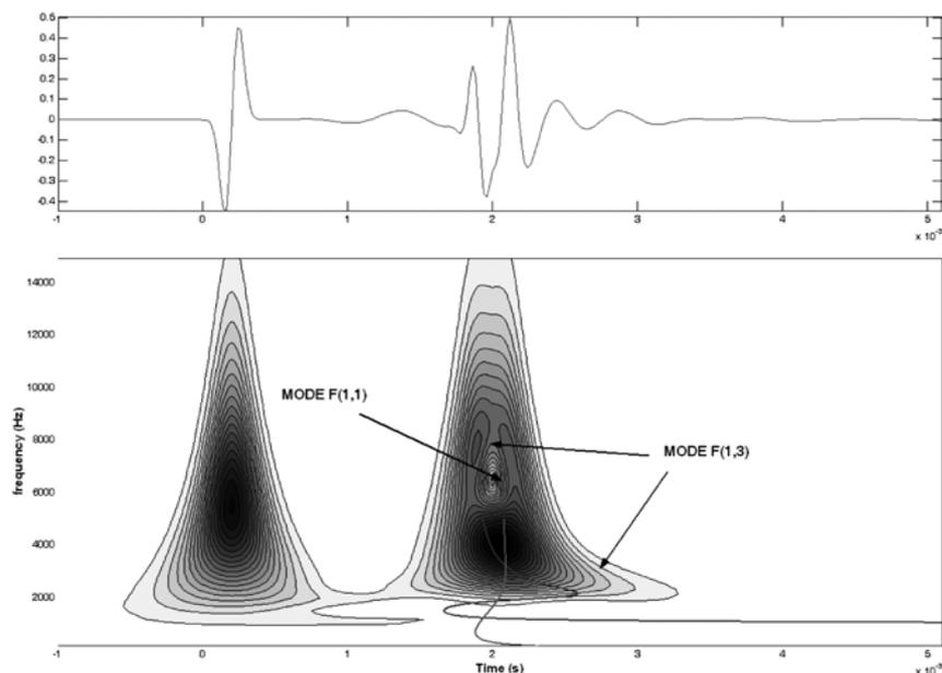
Fig. 11 – Wavelet analysis of a bi-modal signal numerically propagated in a cylinder. Cylinder and signal properties as above. Gabor wavelet with  $\sigma=1$  and  $\eta=5$ .
