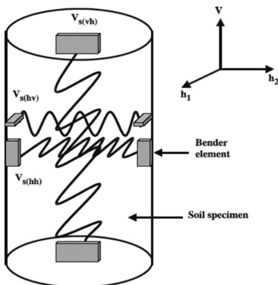
Fig. 2 – Example of a laboratory pulse test configuration (from PENNINGTON *et al.*, 1997).
