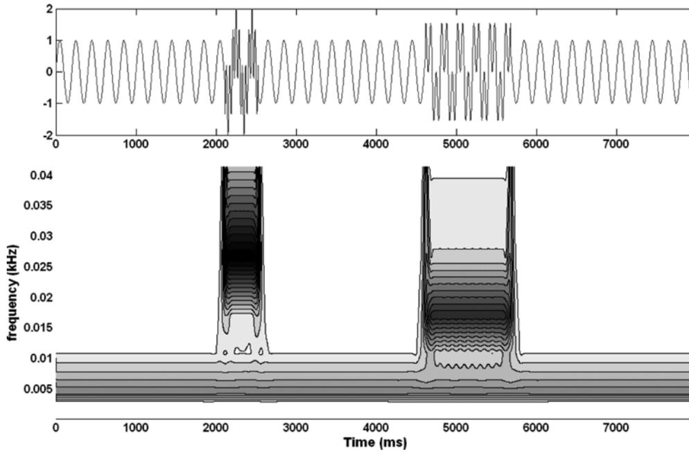
Fig. 6 – Normalised scalogram of an harmonic signal of basic frequency  $f = 5$  Hz with two superimposed signals of frequency  $5*f$  (at time 2.11 to 2.53 s) and  $3*f$  (at time 4.62 to 5.68). Gabor wavelet with  $\sigma = 1$  and  $\eta = 5$ .
