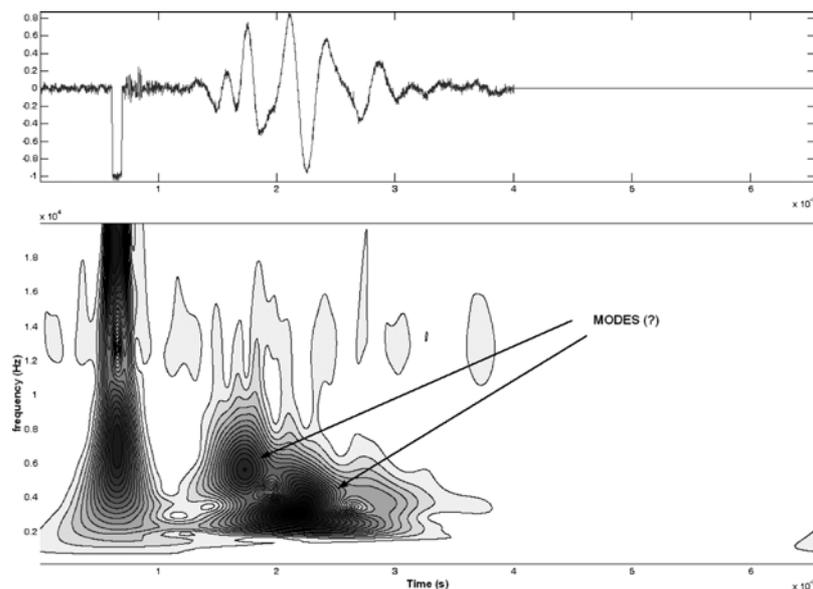
Fig. 12 – Scalogram of an input pulse signal and its response in a through transmission test in reconstituted Gault clay. 121 mm transmission distance, 6 kHz apparent pulse frequency. Gabor wavelet with  $\sigma=1$  and  $\eta=5$ .
