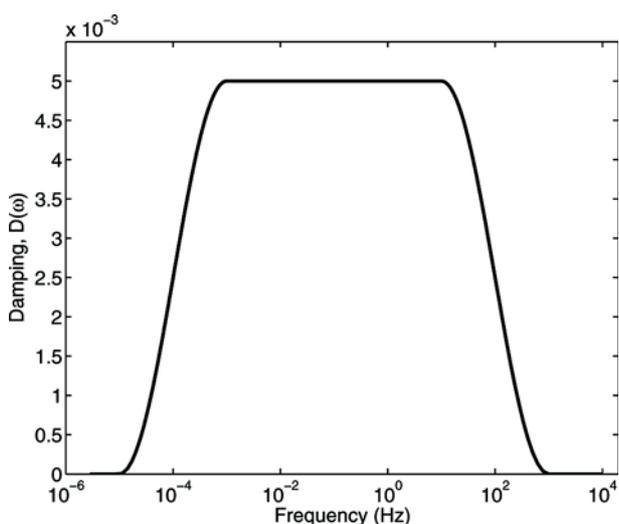
Fig. 5 – Theoretical model constructed for frequency-independent (i.e. hysteretic) damping ratio over the seismic band of 0.001–10 Hz.
