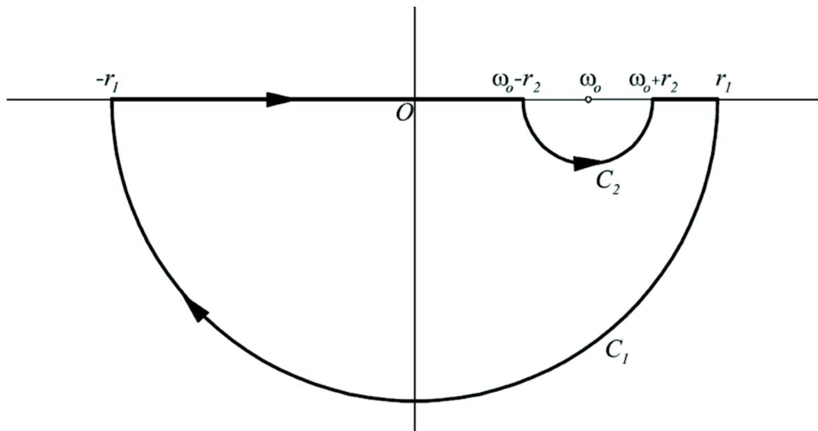
Fig. 3 – Closed contour in the lower part of the complex plane used for the derivation of the Kramers-Kronig relations from the analyticity and boundness of the complex modulus [from MEZA-FAJARDO, 2005].
