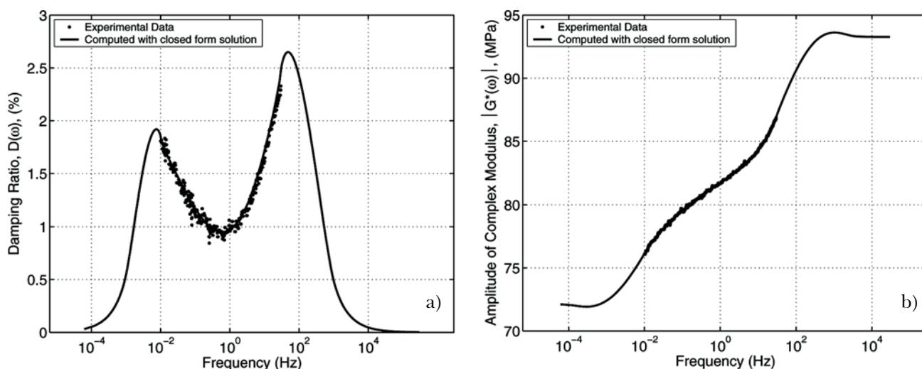
Fig. 10 – Comparison between experimental data obtained by RIX and MENG [2005] in applying the non-resonant column testing method to remoulded kaolin and theoretical predictions from Eqs. (21b) and (23) [from MEZA-FAJARDO and LAI, 2006].
