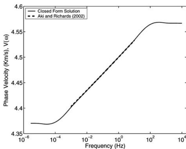
Fig. 6 – Comparison of phase velocity dispersion curves obtained for rate-independent (i.e. hysteretic) damping ratio using exact and approximate solutions. The exact solution has been calculated via Eq.(27) adopting the damping ratio function shown in Fig. 5. The approximate solution has been determined using Eq.(16).
