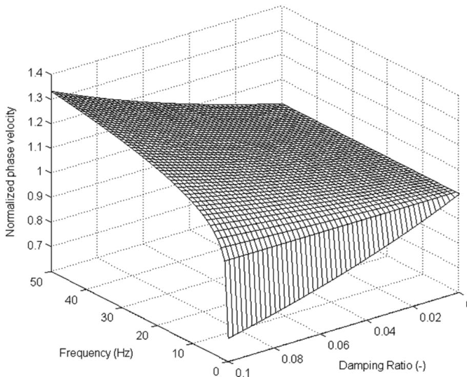
Fig. 4 – Frequency-dependence of phase velocity of viscoelastic bulk waves predicted by the dispersion relation represented by Eq.(16) and based on assuming rate-independent (i.e. hysteretic) material damping ratio over the seismic frequency band.
