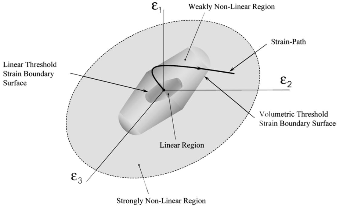
Fig. 2 – Conceptual illustration of mechanical response of geomaterials to a dynamic excitation in *multi-axial* loading. Dependence of response on the *norm* of the deviatoric strain tensor shown through the concepts of linear and volumetric cyclic threshold strain boundary surfaces in the principal strain space [from LAI, 2005].
