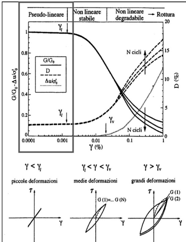
Fig. 1 – Qualitative illustration of mechanical response of geomaterials to a dynamic excitation of cyclic simple shear (*uniaxial* loading). Dependence of the response on the magnitude of the shear strain in relation to the concepts of linear  $\varepsilon^l$  and volumetric  $\varepsilon^v$  cyclic threshold shear strain [from SILVESTRI, 2005].
