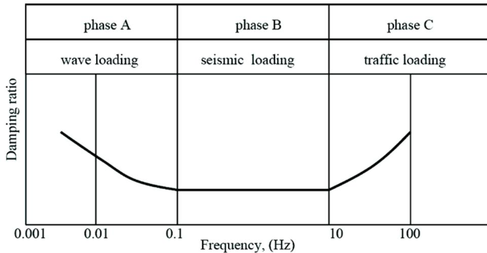
Fig. 7 – Qualitative description of the frequency-dependence of small-strain, damping ratio in fine-grained soils [after SHIBUYA *et al.*, 1995].
