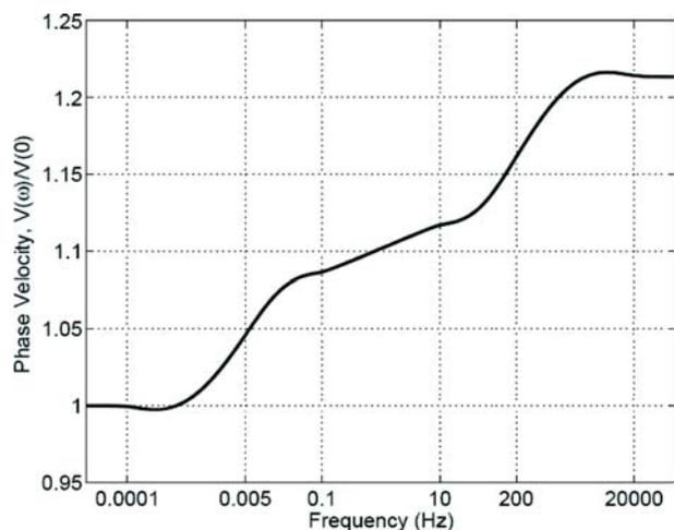
Fig. 9 – Phase velocity dispersion curve obtained from Eq. (27) using the damping ratio function  $D(\omega)$  shown in Fig. 8.
