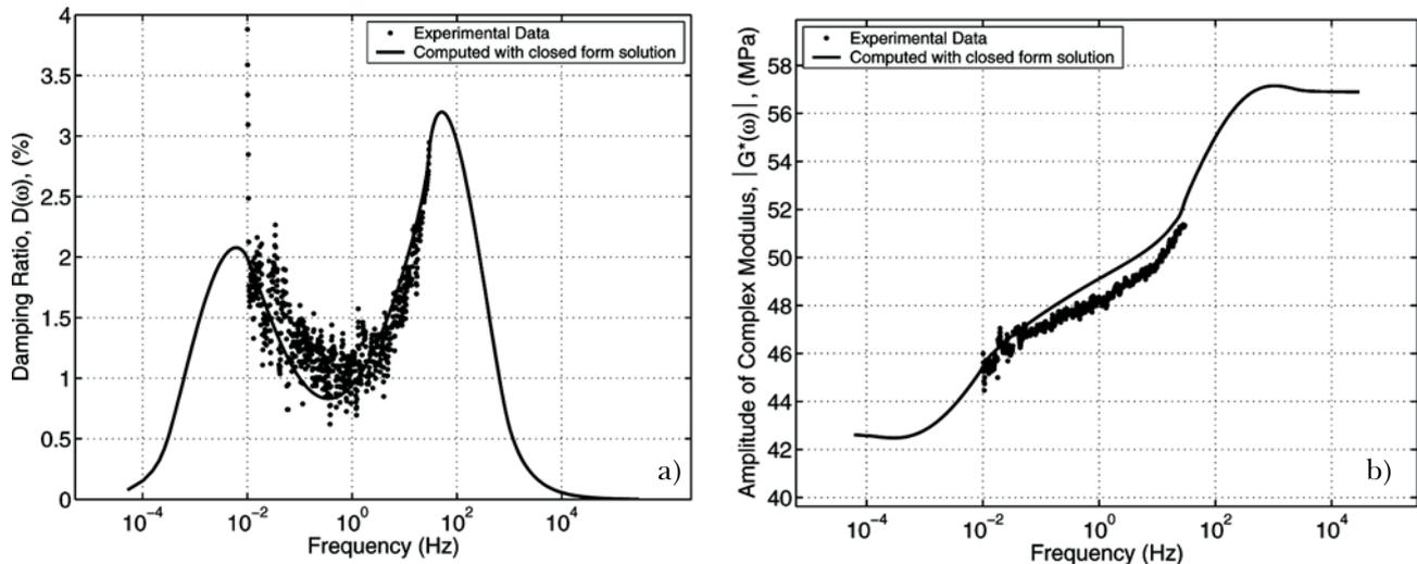
Fig. 11 – Comparison between experimental data obtained by RIX and MENG [2005] in applying the non-resonant testing method to natural sandy silty clay and theoretical predictions from Eqs. (21b) and (23) [from MEZA-FAJARDO and LAI, 2006].
